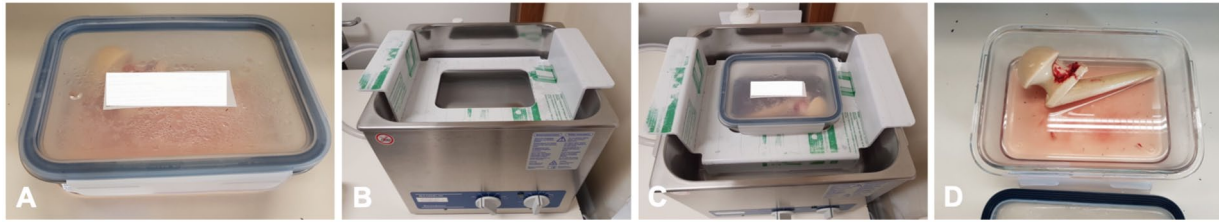
Fig. 4 (A) Implant (in this case a hip spacer) sent to the laboratory in a solid container with airtight seal; (B) sonicator at the laboratory bench; (C) sonication of the container with the implant; (D) only after sonication is the container opened using aseptic technique and sonication fluid is collected and inoculated into selected culture media.
