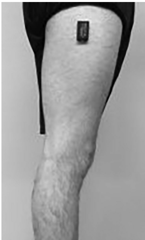
Fig. 1 An accelerometry-based activity sensor worn laterally on the thigh.
