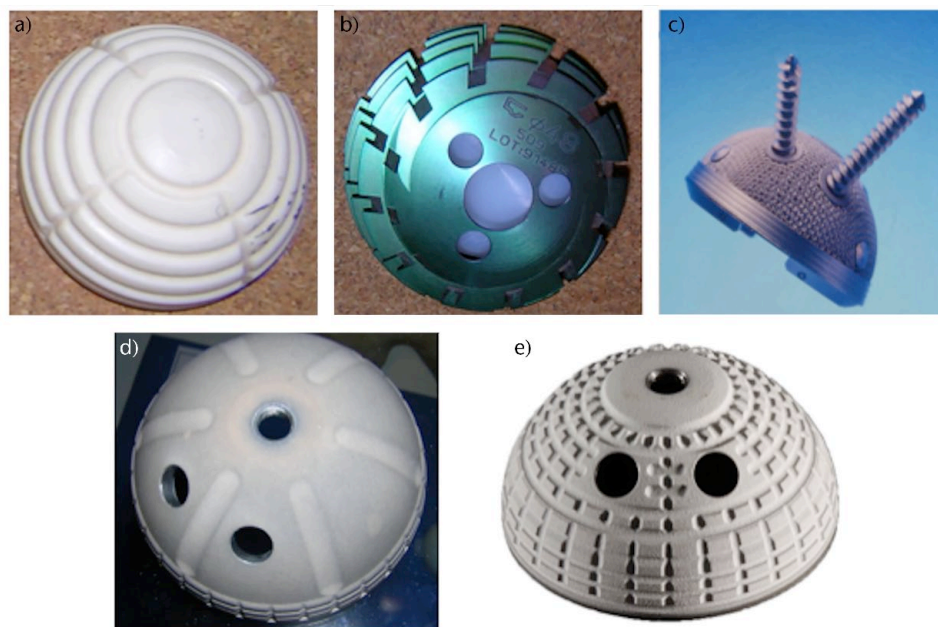
Fig. 1 The design of the acetabular component has been modified over the last 40 years: a) impacted or cemented plain alumina socket; b) smooth titanium screwed-in shell with alumina liner; c) press-fit titanium shell with titanium grid; d) hydroxyapatite-coated titanium shell; e) hydroxyapatite-coated titanium shell entirely covered with a microstructure of ridges and grooves.
